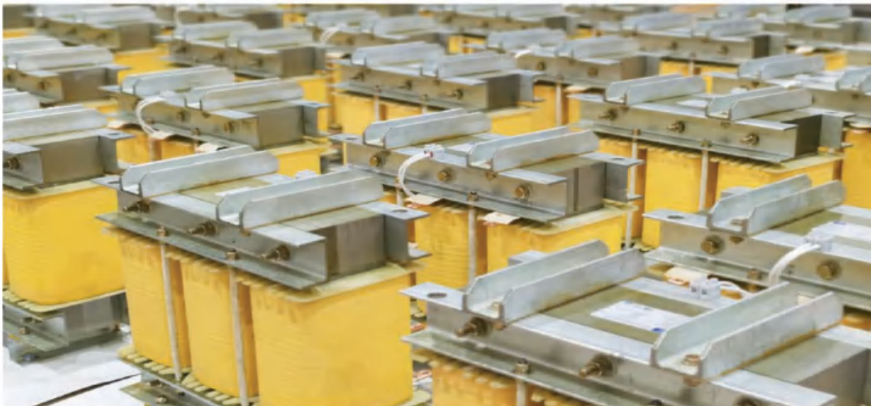
Filter reactors for 690V 200kVar capacitors in 480V system to limit the 3 harmonics
