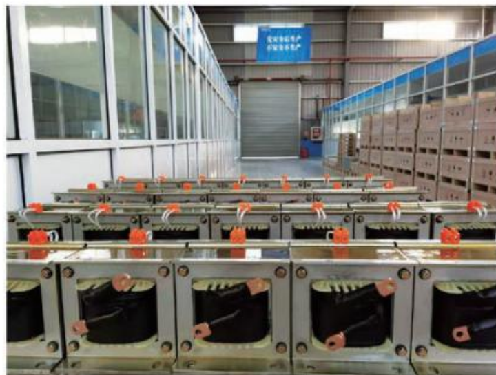
Single phase reactors for traditional compensations in Chinese networks
